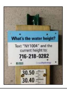
CrowdHydrology sign and gage plate ready to mount on the pressure treated board using 1.25" screws
